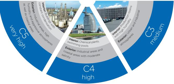
The corrosivity categories were restructured in the 2018 revised standard and now range from C1 to CX. CX describes extreme conditions related to marine climate or tropical atmosphere and is treated within the new part 9 of the standard.
