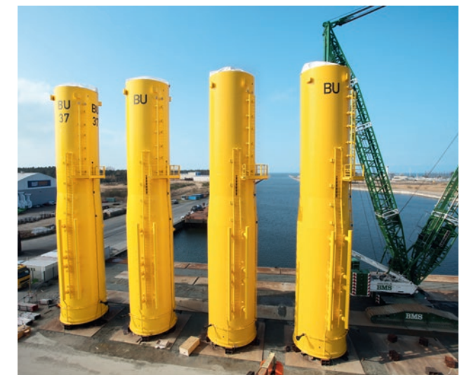
Transition pieces Windfarm Butendiek
