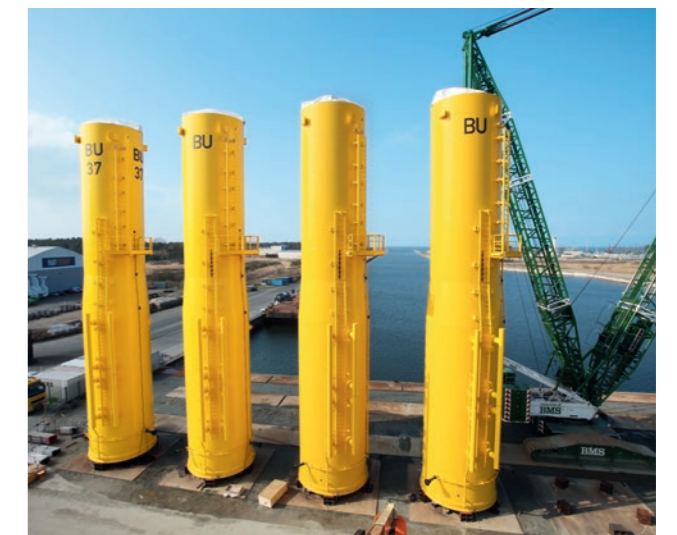
Transition pieces Windfarm Butendiek
