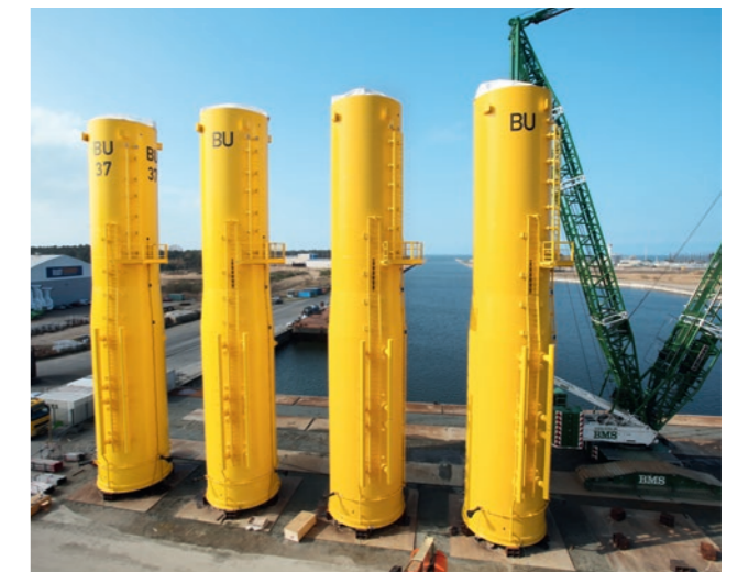
Transition pieces Windfarm Butendiek
